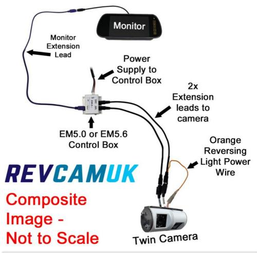
Overview of the twin reversing and rear view camera system installed on a lot of Swift and Autotrail Motorhomes
