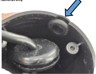
Take the connector from the camera and feed this through the hole you produced in step 3. If you drilled it large enough for the grommet to fit, install this in to position too.
