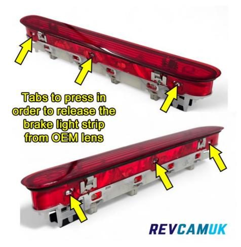
3. Using either a small flat head screw driver or a trim removal tool, press the metal spring clips so that the lens is released from the brake light strip. Work one at a time and apply pressure in between tabs to prevent them reclipping in.
