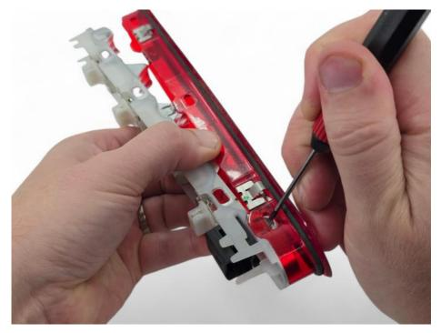
4. Line up the OEM brake light on top of our brake light reverse camera, ensuring the cable is located in the cut-out/groove, and that the tabs line up, see image below.
