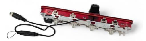
5. Insert the complete unit back in to the original location on the van.
