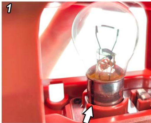
1 - Line up "pins with groove"
